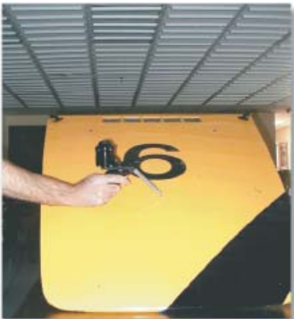
Digitizing with the HiBall-3100 Tracker
